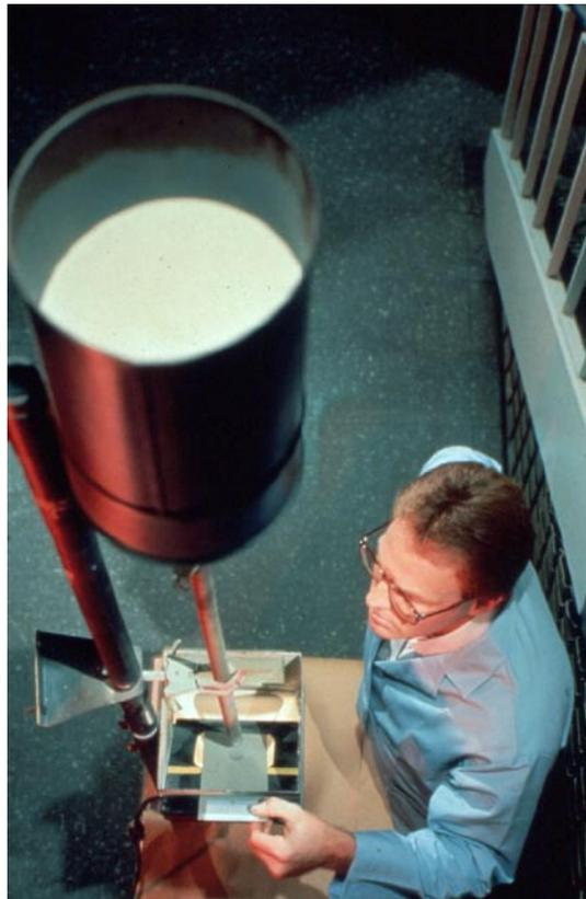
**Figure 7 - Falling Sand Abrasion Test**
