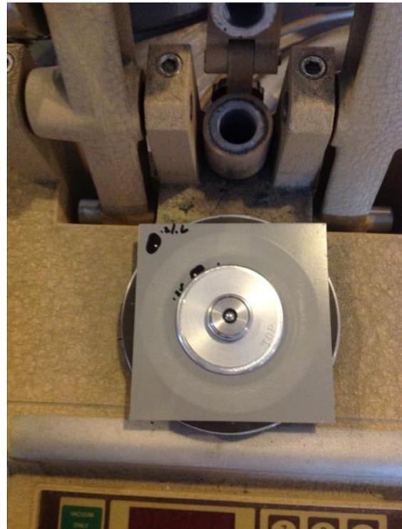
**Figure 8B - Sample Mounted on Taber Abrader**
