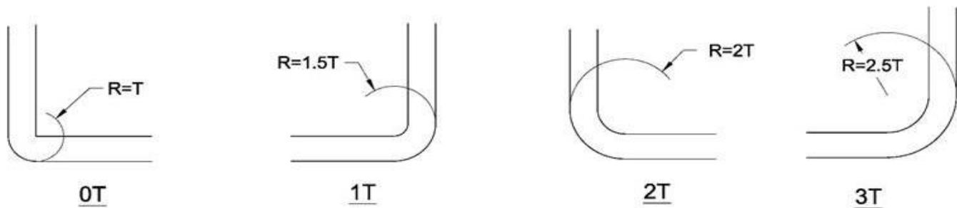
It can be important to know the amount of stretching that takes place at the outer layer of metal being fabricated, since this stretching is what the paint experiences during fabrication. It also may be important to calculate the T-bend equivalent of a bend, based on the inner radius of the bend and the metal thickness. A few equations may be used that describe this information (see **APPENDIX** for additional information):
