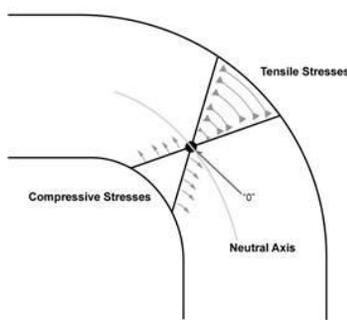
When testing the flexibility of prepainted metal, a T-bend test is routinely done. The figure below shows typical T-bends using NCCA nomenclature, where T is the thickness of the metal. The inner and outer bend radii are shown in the table below.
