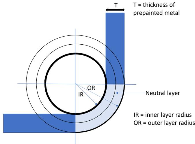
To understand how much elongation takes place at the outer layer, calculate the strain at the outer layer, where strain,  $\epsilon$ , is the change in length at the outer layer, divided by the original length. The neutral layer—that layer that does not change its length during fabrication—is used as the original length of the outer layer before fabrication.
